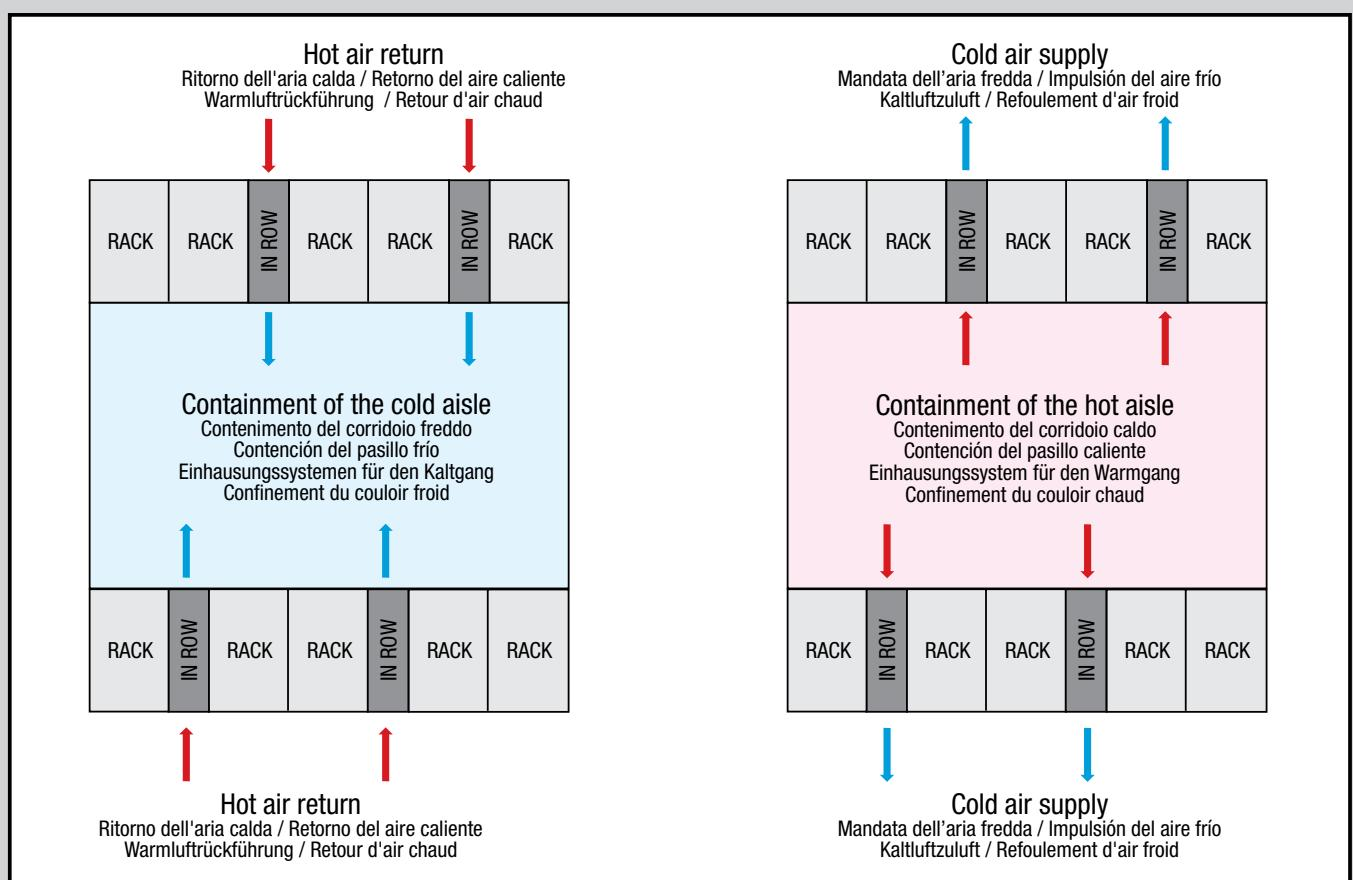
With containment on the cold aisle, using front delivery machines will be sufficient, whereas using the lateral delivery will be evaluated in the case of containment of the hot aisle. When there are multiple rows of racks, it is always advisable to never align the different unit deliveries belonging to the same aisle with each other, to obtain better air distribution (see the figure on page 45).
